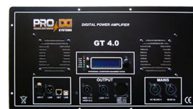
GT 4.0 1 canal / channel 2500 W graves / LF. 1 canal / channel 900 W medios / MF. 1 canal / channel 900 W agudos / HF.
